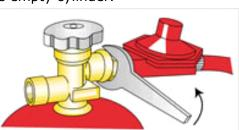
5. Replace the protective plug into the valve outlet
