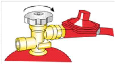
1. Turn the handwheel OFF (clockwise rotation). Wait until the burner/pilot light has gone out
