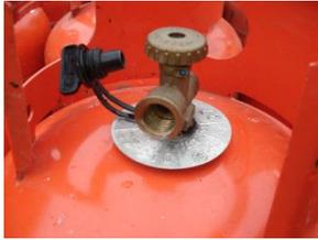
1. Check that the valve handwheel is OFF by turning clockwise
